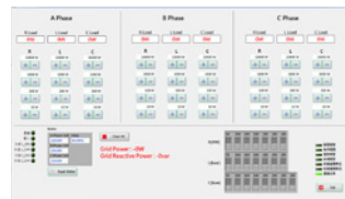
RLC Load Control Test
