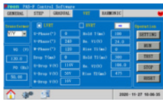
Low Voltage Ride Through Setting
